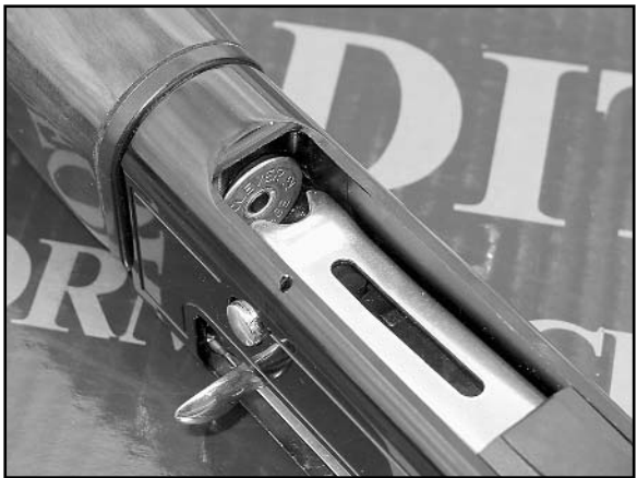
Easy loadin'. The ALS 2100's shell carrier stays half-depressed between shots, forming a kind of "shell well." It's one of the easiest designs to speed-reload this side of a Mossberg pump.
